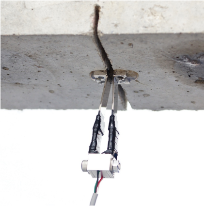
CMOD test arrangement
